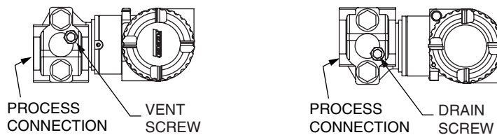
Figure 21. Horizontal Mounting - Cavity Venting and Draining
